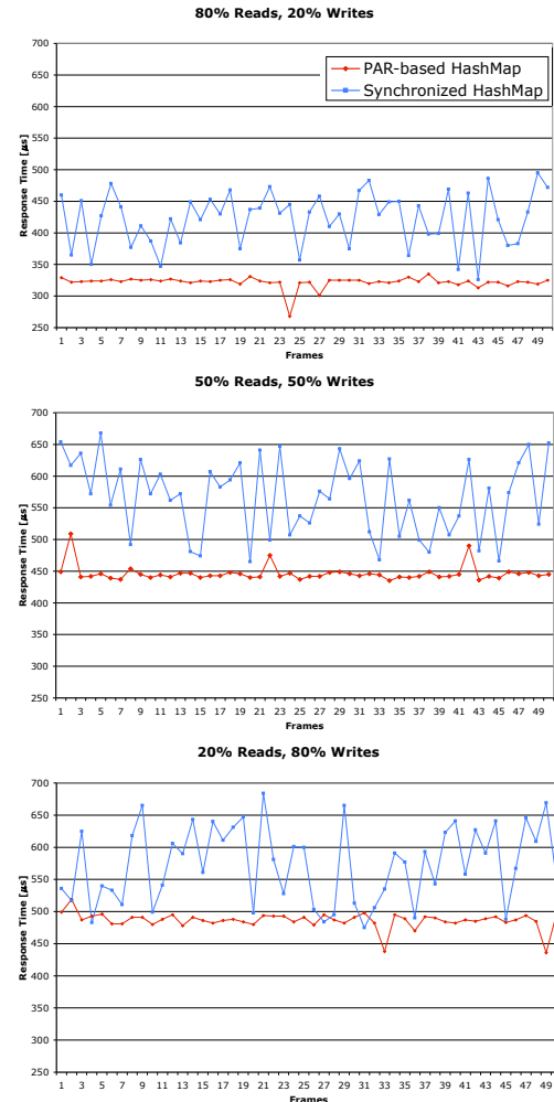
Figure 4. Response time of a high-priority thread in the HashMap Microbenchmark. The x-axis indicates the number of periods that have elapsed (frames), and the y-axis indicates the response time of the high-priority thread (in microseconds). Lower is better. The graph compares RTSJ locks with PARs, and indicates that using PARs provides consistently better performance.
